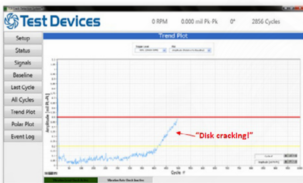
Figure-5: Example of Real-Time Crack Detection data.
