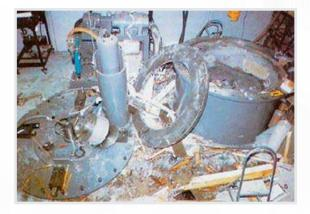
Fig. 3 – The spin pit cover with stripped retaining bolts is lying on the floor next to the spin chamber after the accident. The explosion destroyed the chamber and made holes in the wall and roof of the building where the experiment was being conducted.
