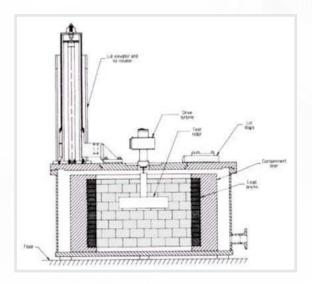
**SPIN TEST SYSTEMS**, which are used extensively in the turbomachinery industry for evaluating the centrifugal strength and fatigue life of high-speed rotating components such as turbine disks and centrifugal compressors, allow stress testing of high-speed components in a controlled environment. Therefore, these systems are faster and less expensive to use than testing in the target engine or machine.
