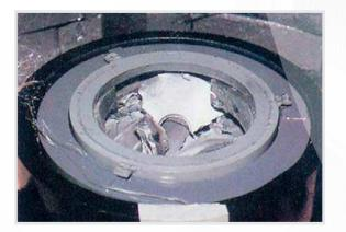
Fig. 3 – To solve the problem, a ledge that would cause the lead to fold back harmlessly into the pit was designed. The model spin pit inside a larger test pit is shown immediately following a lead extrusion containment burst. All the lead was contained inside the pit after the test.
