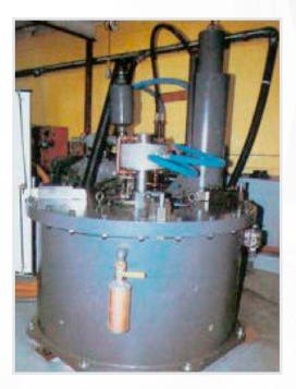
**SPIN TEST SYSTEMS**, which are used extensively in the turbomachinery industry for evaluating the centrifugal strength and fatigue life of high-speed rotating components such as turbine disks and centrifugal compressors, allow stress testing of high-speed components in a controlled environment. Therefore, these systems are faster and less expensive to use than testing in the target engine or machine.
