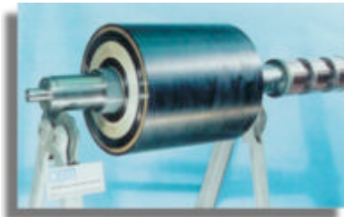
Figure 2 Engineers at the Center for Electromechanics developed this high-performance, 2-kilowatt-hour, 150-kilowatt, 40,000-rpm flywheel rotor that will be used in a future hybrid electric transit bus.
