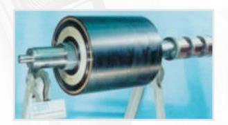
Fig. 2 – Engineers at the Center for Electromechanics developed this high performance, 2-kilowatt-hour, 150-kilowatt, 40,000-rpm flywheel rotor that will be used in a future hybrid electric transit bus.
