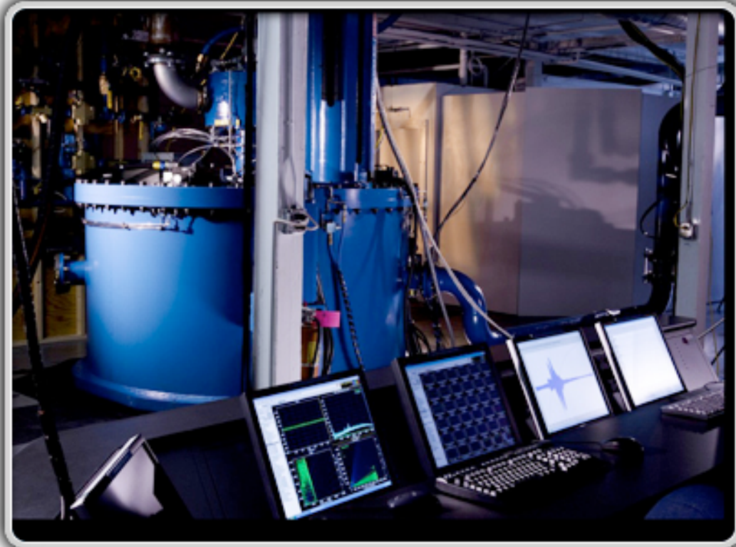
Figure 1 Test Devices Inc.'s strain gauge and non-intrusive stress measurement instrumentation stations are part of the aero-pulse high cycle fatigue spin test system at its facility in Hudson, MA.
