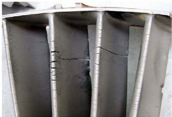
Figure-6 – Cracked and Ruptured Blade (Courtesy of [6]).
