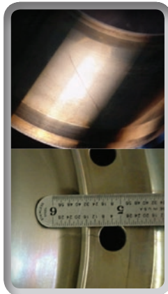
Figure 1 – Cracks detected using Test Devices' Crack Detection system
