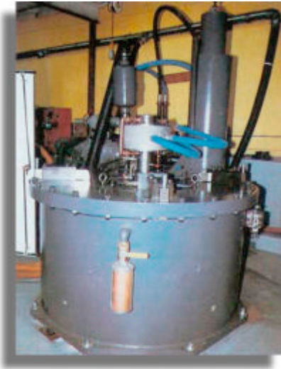
Figure 2 This 36" spin test system was used by Test Devices Inc. to burst a rotor and demonstrate that the containment structure would satisfactorily support the event (see "Anatomy of an Accident"). However, the system, which included a spin chamber, turbine - atop the pit with two blue hoses entering the side - and vacuum and oil pumps, was later destroyed in an accident.
