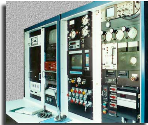
Figure 3 Modern Spin Test Console with Vibration Monitor, Heated Test Capability, Tachometer, PC Computer Interface, Slip Ring System and Radio Telemetry for Strain Measurement and High Speed Camera Control
