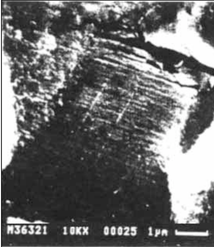
Figure 8 Scanning Electron Micrograph showing striations detected near a crack origin in the HPT assembly.
